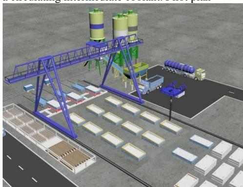
**Fig.2.** Diagram of an open heliopoly of polystyrene concrete products
