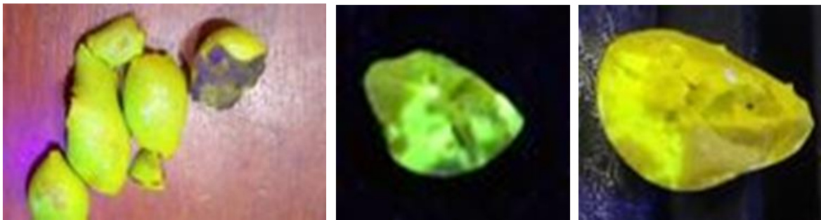
Figure 1. Photographs of samples of synthesized YAG: Ce ceramics illuminated by white light (the first picture) and excited by LED radiation (next two pictures)
