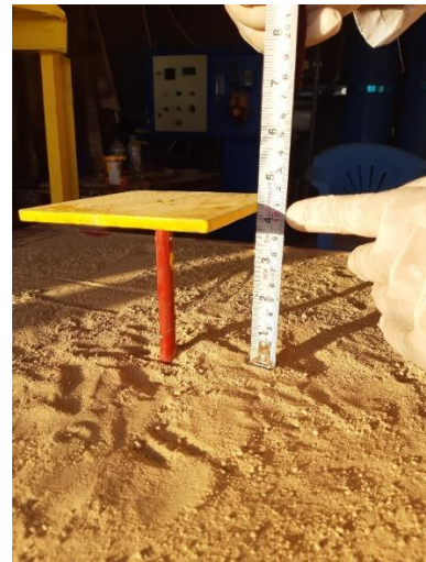
Figure 7. Gap between pile cap and soil surface.
