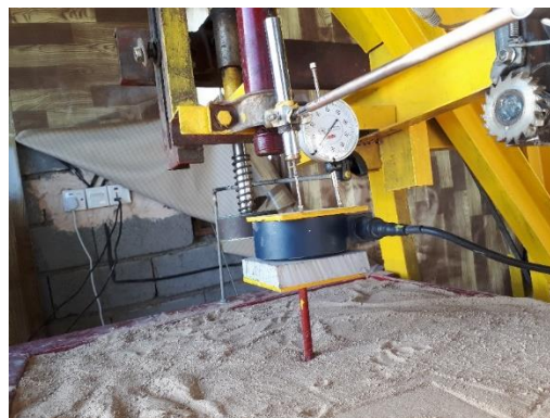
Figure 8. Loading system of screw pile and gauges.
