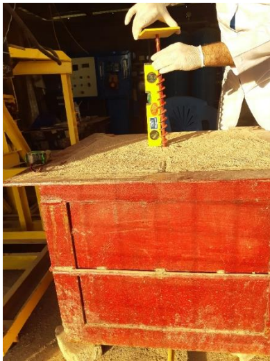
Figure 6. Insertion of screw pile in soil.
