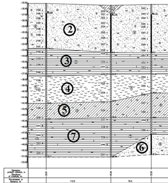
Fig.2 Geotechnical cross-sections on the construction site on Tengiz
