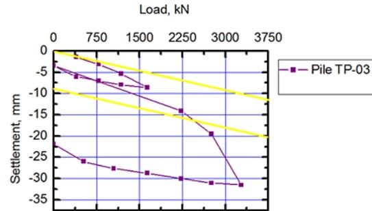
Fig. 9 Results of SCLT pile number TP-03 in construction site “Prorva”
