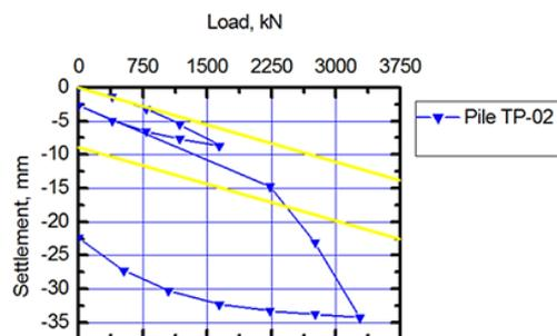
Fig. 8 Results of SCLT pile number TP-02 in construction site “Prorva”
