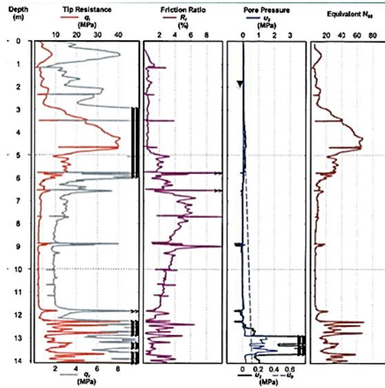
Fig.1 CPT on the construction site on Tengiz
