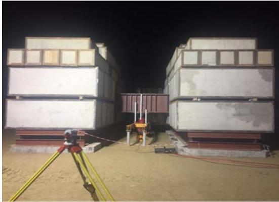
Fig. 5 The testing platform for static compression load test (SCLT) in site "Prorva"
