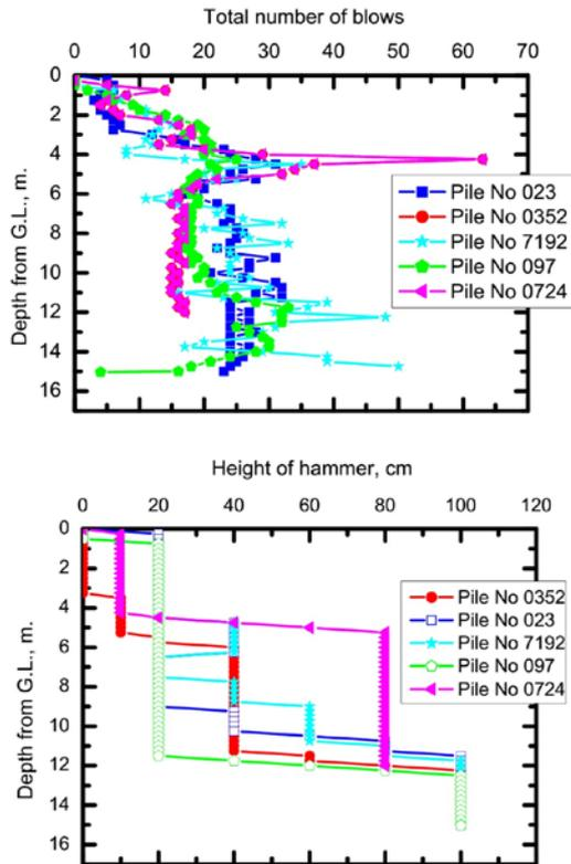
Fig. 3 Driving records of piles on site on Tengiz
