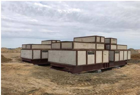
Fig. 6 Static load test system in construction site Tengiz
