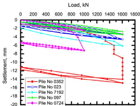
Fig. 10 Load and settlement curves of piles in construction site on Tengiz
