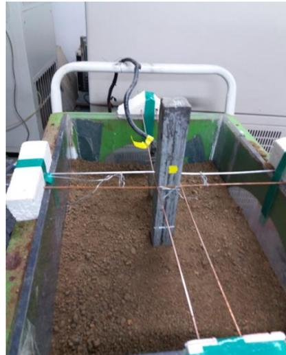
Fig. 3 Model of pile foundation in the Model Test Box (MTB)
