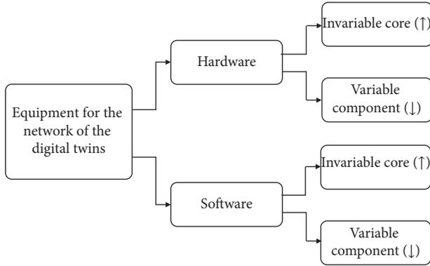
FIGURE 8: Decomposition of equipment for the network of digital twins.
