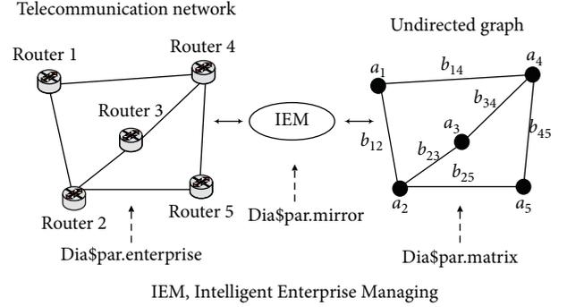
FIGURE 6: Digital twin creation for telecommunication network.
