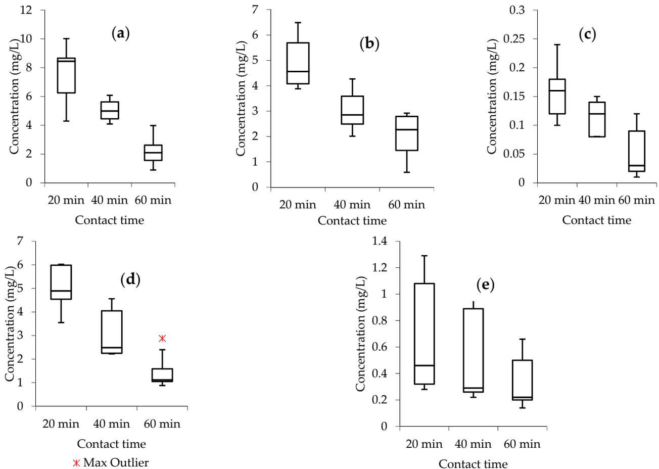
**Figure 7.** Boxplots for potentially toxic elements, (a) total iron, (b) aluminum, (c) manganese, (d) nickel, (e) chromium.
