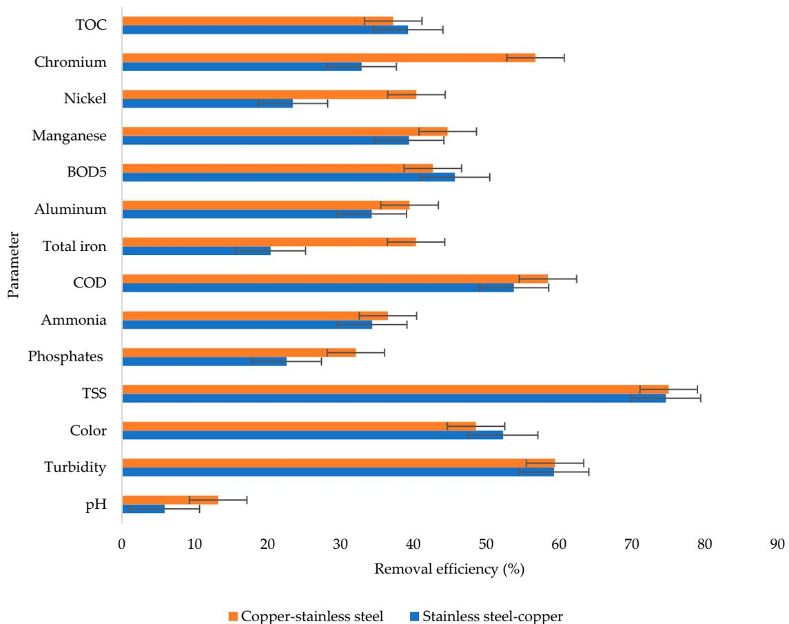
**Figure 8.** Removal efficiencies from 20-min contact time.
