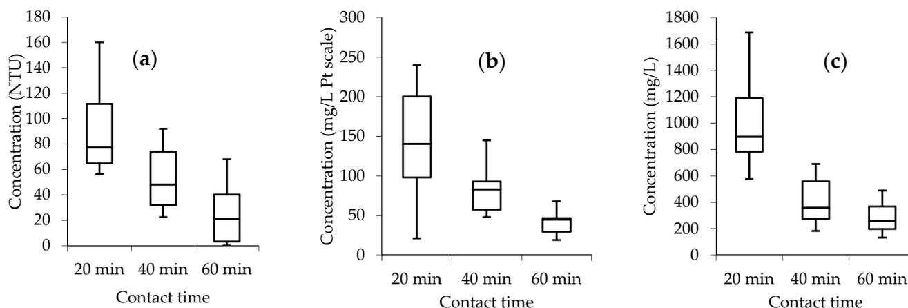
**Figure 4.** Data distribution for some physicochemical parameters after treatment, (a) turbidity, (b) color, (c) TSS.
