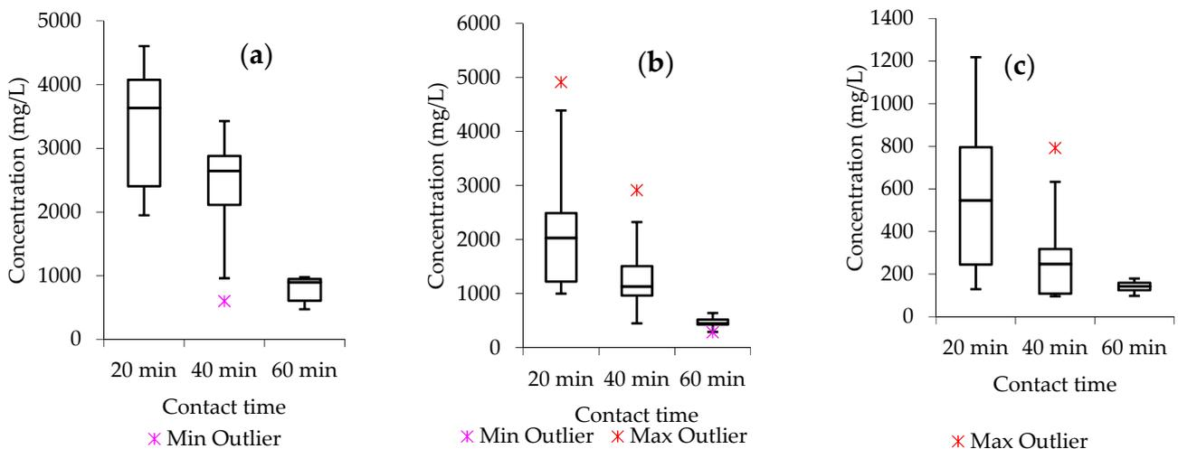
**Figure 6.** Data distribution for organic-related parameters in the treated effluents, (a) COD, (b) BOD, (c) TOC.
