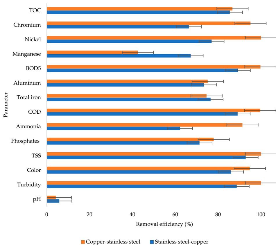
Figure 10. Removal efficiencies from 60-min contact time.
