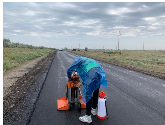
Fig.4 Sampling process for pavement materials
