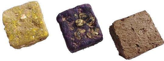
Fig.5 Samples of pavement materials for the thermo-technical test
