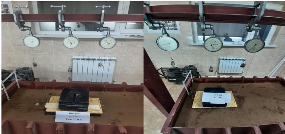
Fig. 4. Static tests of the DDS and CFA model piles
