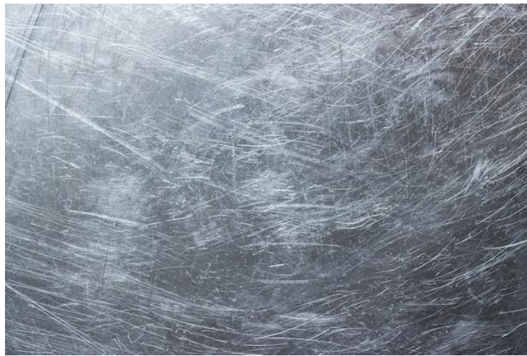
Figure 2. Sinks with traces of wear ("false brining")
