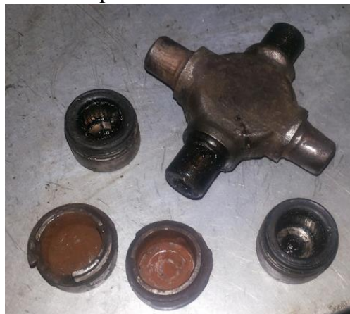
Figure 3. The appearance of worn parts ("false brining") of the bearing assembly of the crosspiece
