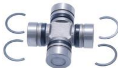
Figure 4. The upgraded crosspiece of the VAZ "Niva" car
