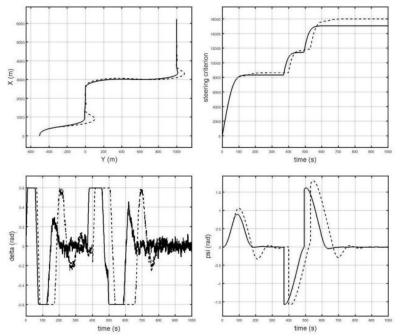
Figure 1. An example outcome of the comparison of the proposed adaptive system (continuous line) and linear quadratic regulator (LQR) regulator without model parameter identification (dashed lined).
