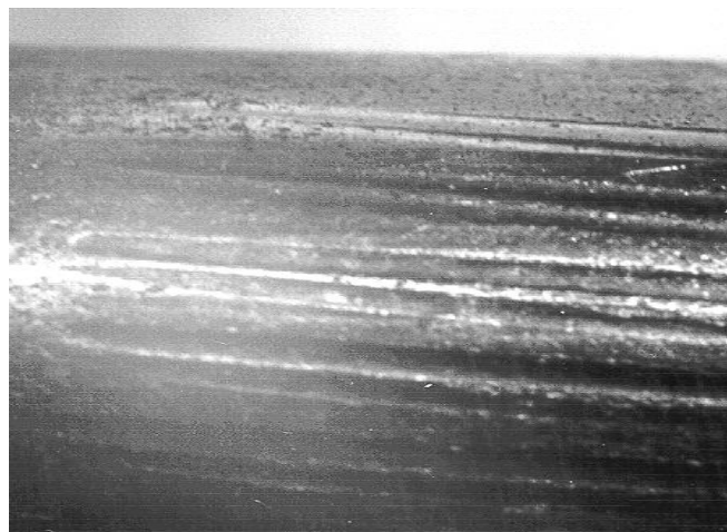
Figure 2. Sinks with traces of wear ("false brining")
