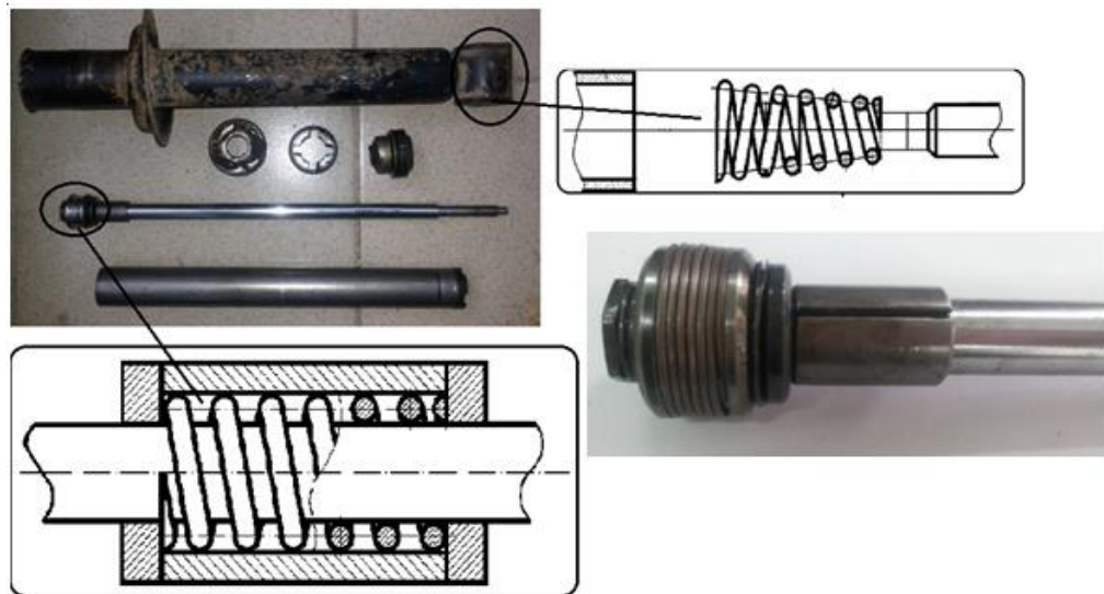
Figure 5. The rear shock absorber of the VAZ 2108 car: the design of a piston with a seal made of a square-section helical cylindrical spring with preloaded coils
