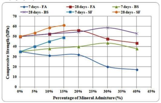
Fig. 1. Compressive strength of LWC with different MA.
