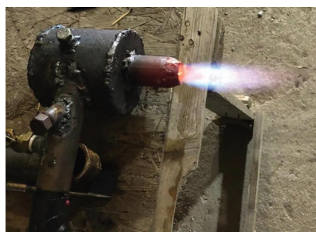
FIGURE 2: Swirl burner device in operation.
