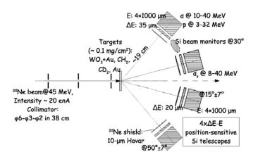
Figure 1: Schematic view of the experimental setup.
