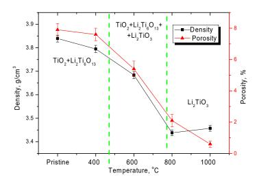
Figure 4. Graph of changes in density and porosity of ceramics depending on annealing temperature.
