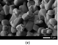
Figure 1. SEM images of synthesized ceramics: (a) pristine; (b)  $400 \degree C$ ; (c)  $600 \degree C$ ; (d)  $800 \degree C$ ; (e)  $1000 \degree C$ .
