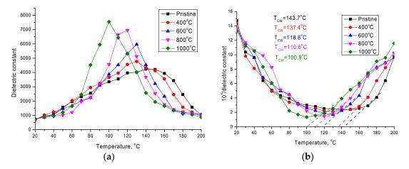
Figure 6. (a) Graph of changes in the dielectric constant; (b) graph of inverse dielectric constant and Curie–Weiss temperature.
