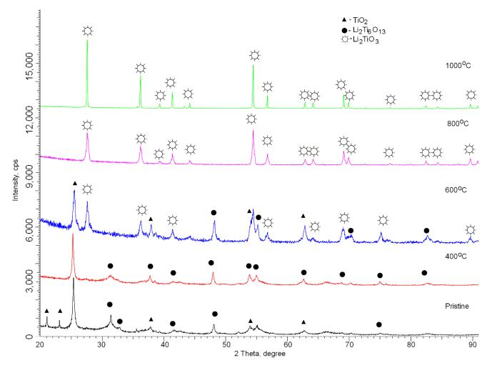
Figure 2. Results of X-ray diffraction of lithium-containing ceramics.
