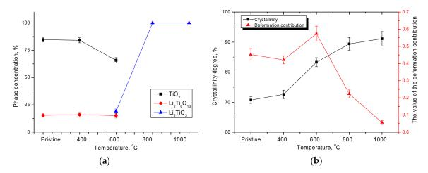
**Figure 3.** (a) Diagram of ceramic phase composition depending on annealing temperature; (b) graph of changes in the crystallinity degree and deformation contributions to the change in the shape of diffraction reflections.
