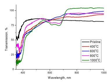
**Figure 5.** UV-Vis transmission spectra of synthesized ceramics depending on the change in annealing temperature.
