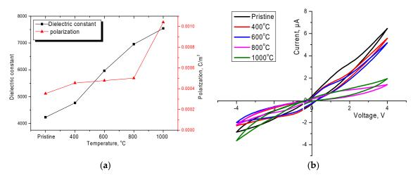
**Figure 7.** (a) Graph of the change in the dielectric constant maximum and spontaneous polarization; (b) graphs of cyclic volt-ampere characteristics of ceramics.
