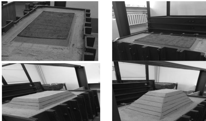
Figure 4. Layered laying of a dam model without reinforcement.
