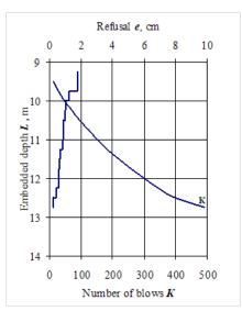
Fig. 10 Graphics after pile length increasing, LT4
