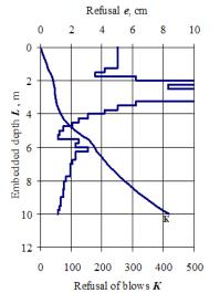
Fig. 5 Graphics before pile length increasing for testing pile LT3
