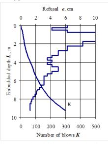
Fig.6 Graphics before pile length increasing for testing pile LT4
