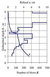
Fig. 3 Graphics before pile length increasing for testing pile LT1
