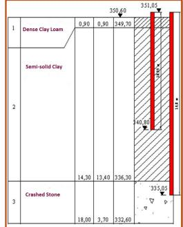
Fig. 2 Geology of the construction site of the USA Embassy in Astana
