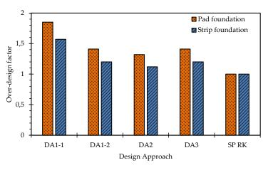
**Figure 7.** Comparison of the values of over-design factor for pad and strip foundations adhering to Kazakhstani and European approaches.
