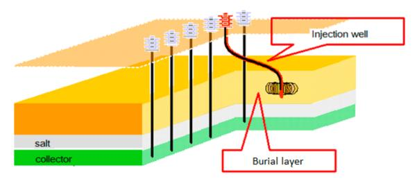
Figure 2. Scheme of injection of drill cuttings in the underground horizon.
