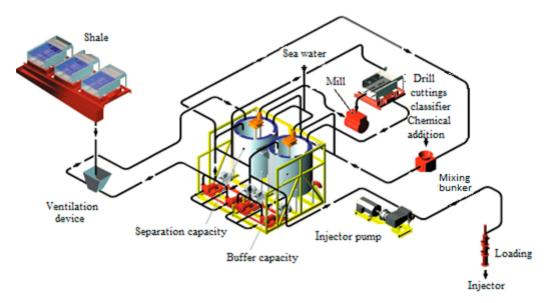
Objects of ground equipment of the drilling sludge injection system of the considered technology and the option of utilization of drilling sludge can be represented as a Figure 1.
