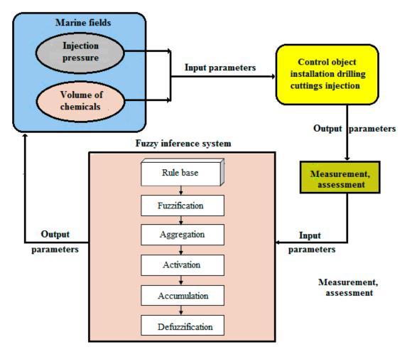
Figure 3. The structure of the elements of the fuzzy inference system.
