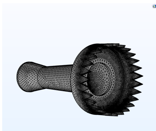
Figure 9. Adaptive computational grid of the simulated area in COMSOL Multiphysics
