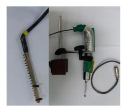
Fig.5Thermocouple T type and LVDT
