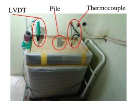
Fig.1 The photo of Model Test Box
