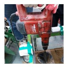
Fig.4 Compaction procedure of soil ground
