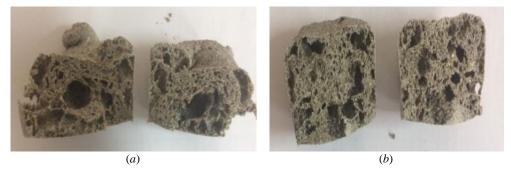
Fig. 3. Samples of polymervermiculite at a ratio of vermiculite: resin 1: 1 (a) and 1: 1.5 (b)
