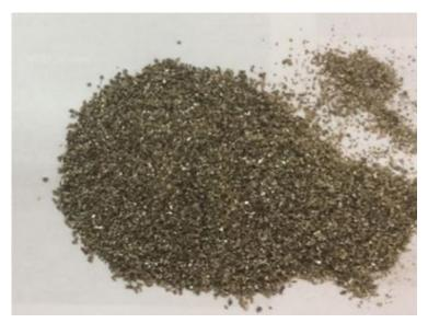
Fig. 1. Vermiculite swelled in the microwave
