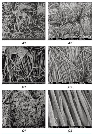
Fig. 2. SEM images of: A1, B1, C1 – untreated fabric and A2, B2, C2 – treated fabric using different magnifications (A1, A2 with 50×, B1, B2 with 100× and C1, C2 with 500×)
