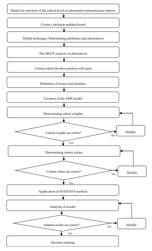
Figure 4. Flowchart of the proposed issue-solving process.
