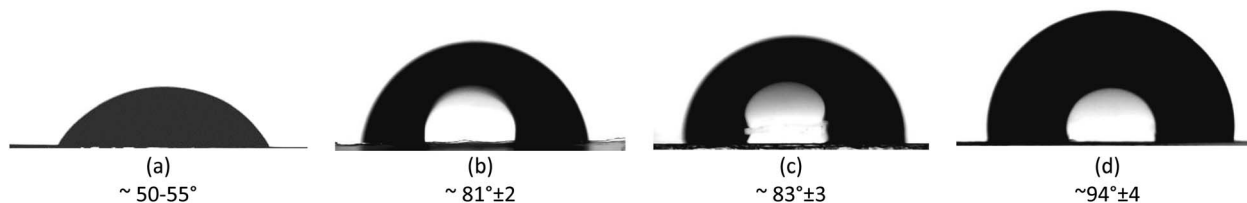
Fig. 7 CA of pristine PET TeM (a) and PET TeMs-g-PLMA with grafting degree of 0.6% (b), 1.74% (c) and 6.84% (d).
