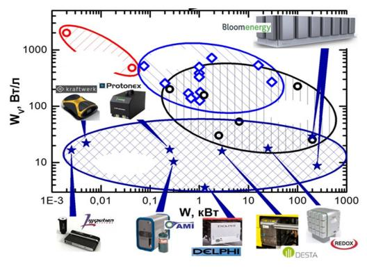
Figure 2. Characteristics of industrial prototypes of SOFC batteries.
