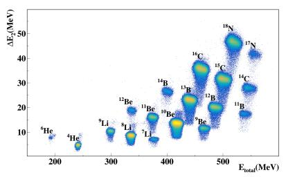
Figure 3. ETwo-dimensional energy spectrum of  $\Delta E_2$  (Si detector 300  $\mu$ m ) and total energy  $E_{total}$ .
