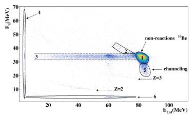
Figure 4. Two-dimensional energy spectrum from detectors  $\Delta E_4$  and CsI(Tl) selected for 33 MeV/nucleon <sup>10</sup> Be incident upon the Si+CsI telescope shown in Figure 2.
