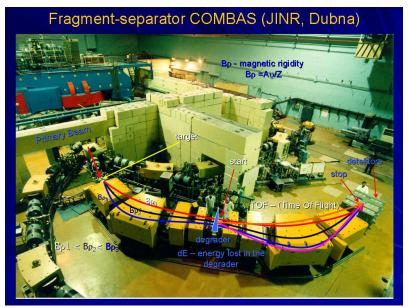
Figure 1. Experimental scheme of the COMBAS fragment separator.
